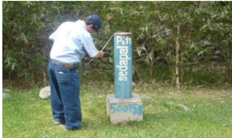
Monitoring of the piezometer network of the Lima aquifer (photo: SEDAPAL S.A.).
