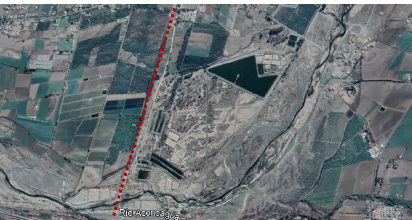
Aerial view of the Aconcagua river, infiltration ponds and water treatment plant. The location of Las Vegas drain is highlighted in red (photo: Google Earth, 2021).
